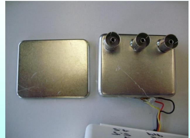
RF amplifier in a shield box
